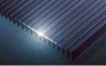
B 采用强光手电对板材横截面进行照射，与板材其它部分相比，UV层会变得更亮许多，仿佛板材表面镀了一道银边，且能清晰的看出UV分布是否均匀。 The UV layer becomes brighter than other part under UV flashlight. You can even see how thick and flat the UV was coextruded through the silver line.
