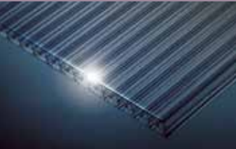
B 采用强光手电对板材横截面进行照射，与板材其它部分相比，UV层会变得更明亮许多，仿佛板材表面镀了一道银边，且能清晰的看出UV分布是否均匀。 The UV layer becomes brighter than other part under UV flashlight. You can even see how thick and flat the UV was coextruded through the silver line.
